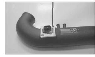
23. Secure the mass air sensor assembly onto the K&N<sup>®</sup> intake tube with the provided hardware.
