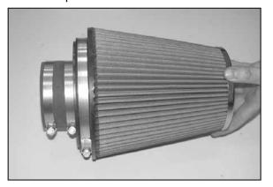
29. Install the filter adapter assembly into the K&N $^{\! \otimes}$  air filter.
