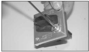
21. Insert the mass air sensor into the mass air sensor adapter and secure with the provided hardware.
