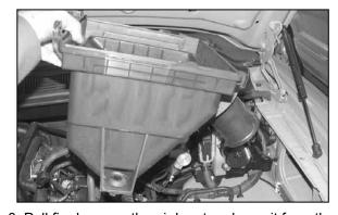
8. Pull firmly up on the air box to release it from the mounting studs, then remove the air box from the vehicle.
