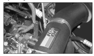
25. Secure the  $K\&N^{\otimes}$  intake tube to the saddle bracket with the provided hose clamp. Also tighten the hose clamp at the throttle body.
