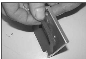
20. Apply the provided gasket to the mass air sensor adapter as shown; sticky side down.
