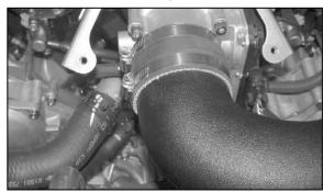
24. Install the K&N® intake tube onto the throttle body and align with the saddle bracket.
