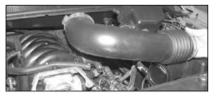
5. Loosen the hose clamps at the throttle body and air box, then remove the intake tube from the vehicle.
