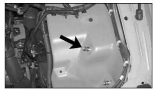
9. Remove the air box mounting stud shown with a 10mm wrench.
