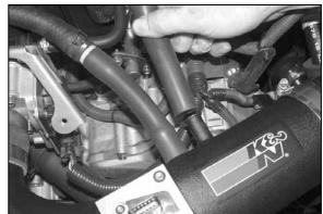
27. Install the provided silicone hose onto the hose mender, then install the hoses onto the intake tube as shown.
