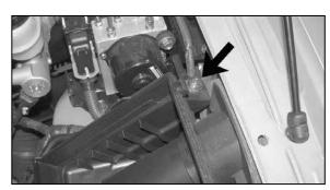
7. Remove the air box mounting bolt with a 10mm socket.
