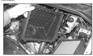
6. Release the two air box lid retainer clips that secure the air box lid to the air box, then remove the air box lid and air filter.
