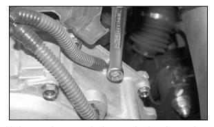
16. Locate the ground wire attached to the engine cam cover and remove the bolt securing it using a 10mm wrench.
